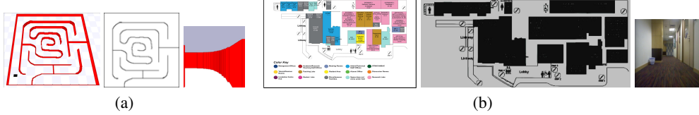
Figure 4: Experimental setup in simulation and real-robot experiments. (a) A simulated environment, the associated 2D map, and a camera view. (b) The floor plan for a robot experiment environment, the occupancy grid map computed from the floor plan, and a camera view of the environment.
